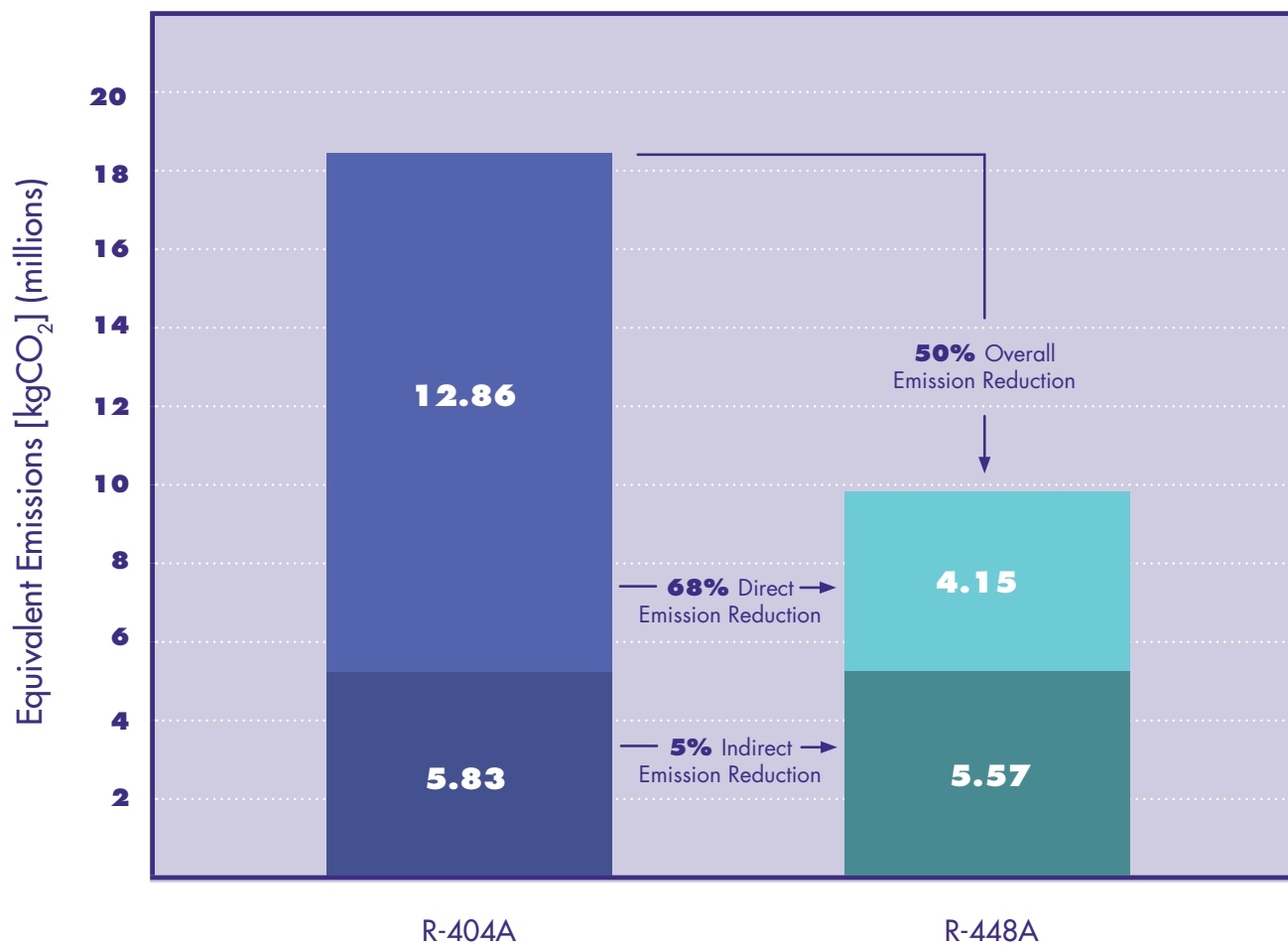
Figure 5: Emission reduction when retrofitting R-404A with R-448A for a 15-year system lifetime in Atlanta, GA
